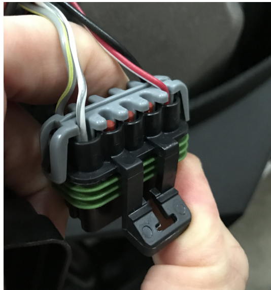
Figure 1. Diagnostic port, AEM installation
